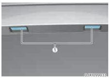
If the LED lamp (1) does not operate, have the system inspected by an authorized retailer of Genesis Branded products.
