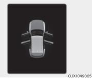
This warning is displayed if any door or hood or liftgate is left open. The warning will indicate which door is open in the display.
