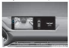
You can change Rear View Monitor settings by pressing the setup icon (♠) on the screen while the system is operating, or select 'Driver Assistance → Parking Safety → Camera Settings' from the Settings menu while the Engine Start/Stop button is in the ON position.
