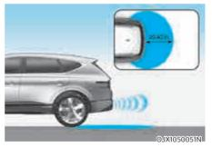
The smart liftgate detecting area extends approximately 20~40 in. (50~100 cm) behind the vehicle. If you are positioned in the detecting area and are carrying the smart key, the hazard warning lights will blink and the chime will sound for about 3 seconds to alert you that the liftgate will open.
