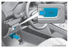
To release EPB (Electronic Parking Brake):
