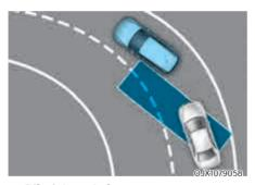
Blind-Spot Safety system may not operate properly when driving on a curved road. The system may recognize a vehicle in the same lane.
