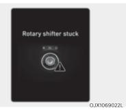
This message is displayed when the shift dial does not return back to it's normal position after rotating it.
