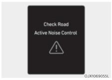
When Road Active Noise Control is not working properly, this warning message will appear on the cluster LCD display. If this occurs, have the system inspected by an authorized retailer of Genesis Branded products.
