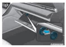
Remove the stoppers on both sides to allow the glove box to hang freely on the hinges.
