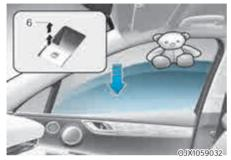
If a window senses any obstacle while it is closing automatically, it will stop and lower approximately 1 in. (2.5 cm) to allow the object to be cleared.
