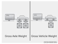
The tongue load is an important weight to measure because it affects the total Gross Vehicle Weight (GVW) of your vehicle. The trailer tongue should weigh a minimum of 10% of the total loaded trailer weight, within the limits of the maximum (15%) trailer tongue load permissible.
