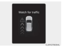
Collision warning when exiting vehicle
