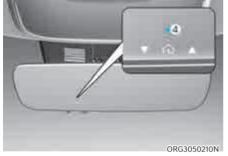
5. If the both indicator (4) and (6) are flashing rapidly for about 5 seconds, the two way synchronization is completed.
