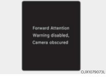
When there is an object right in front of the camera or between the driver and the camera for a certain period of time, Forward Attention Warning will not operate properly, and the 'Forward Attention Warning disabled. Camera obscured' warning message will appear on the cluster.
