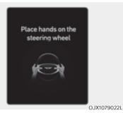
If the driver takes their hands off the steering wheel for several seconds, the 'Place hands on the steering wheel' warning message will appear and an audible warning will sound in stages.
