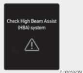
When High Beam Assist is not working properly, the 'Check High Beam Assist (HBA) system' warning message will appear and /\(\Lambda\) warning light will illuminate on the cluster. Have the system inspected by an authorized retailer of Genesis Branded products.
