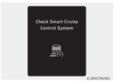
When Smart Cruise Control is not working properly, the 'Check Smart Cruise Control system' warning message will appear, and the \( \underset \) warning light will illuminate on the cluster. Have the system inspected by an authorized retailer of Genesis Branded products.
