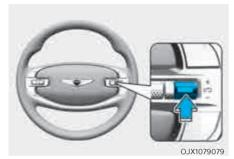
Push the **II** Switch to temporarily pause the set speed limit. The set speed limit will turn off but the Speed Limit (© LIMIT) indicator will stay on.
