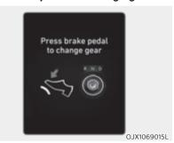
This message is displayed when the brake pedal is not depressed while shifting the gear.
