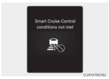
If the Driving Assist MODE button, + switch, - switch or II's switch is pushed when the system's operating conditions are not satisfied, the 'Smart Cruise Control conditions not met' will appear on the cluster, and an audible warning will sound.
