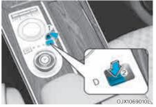
4. Remove the cap-cover (1) and press the button (2) while depressing the brake pedal.
