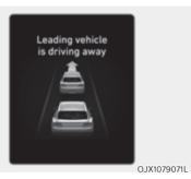
When the front vehicle departs from a stop, Leading Vehicle Departure Alert will inform the driver by displaying the 'Leading vehicle is driving away' message on the cluster and an audible warning will sound.
