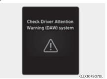
When Driver Attention Warning is not working properly, the 'Check Driver Attention Warning (DAW) system' warning message will appear on the cluster. If this occurs, have the system inspected by an authorized retailer of Genesis Branded products.
