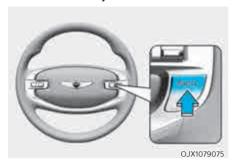
Press the Driving Assist MODE button to turn Manual Speed Limit Assist off. The Speed Limit (MLIMIT) indicator will go off.
