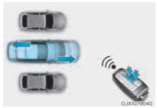
(1) Press and hold one of the Forward (()) or Reverse (()) button on the smart key. Remote Smart Parking Assist will automatically control the steering wheel, vehicle speed and gearshift. The vehicle will move in the direction of the button pressed.
