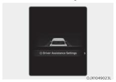
When Driver Assistance Settings menu is selected, press the OK switch on the steering wheel. The 'Driver Assistance' menu will be displayed on the infotainment system screen.
