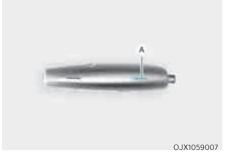
1. Place a soft cloth over the groove (A), and pry open the smart key cover.
