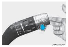
In the OFF position, pull the lever gently toward you to spray washer fluid on the windshield and to run the wipers 1-3 cycles. The spray and wiper operation will continue until you release the lever. If the washer does not work, you may need to add washer fluid to the washer fluid reservoir.
