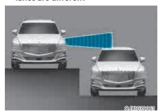
Blind-Spot Safety system may not operate properly when driving where the heights of the lanes are different. The system may not detect the vehicle on a road with different lane heights (underpass joining section, grade separated intersections, etc.). Always pay attention to road and
