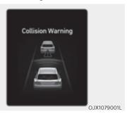
While Smart Cruise Control is operating, when the collision risk with the vehicle ahead is high, the 'Collision Warning' warning message will appear on the cluster, and an audible warning will sound to warn the driver. Always have your eyes on the road while driving, and if necessary, depress the brake pedal to reduce your driving speed in order to maintain a safe distance.
