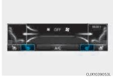
While the engine is running, touch either of the seat warmer icons to warm the driver's seat or front passenger's seat. Manual temperature control
