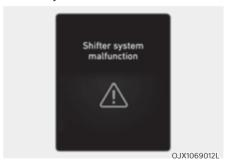
This message is displayed when the transmission or the shift button does not properly operate in the P (Park) position. Immediately have the vehicle inspected by an authorized retailer of Genesis Branded products.
