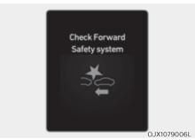
When Forward Collision-Avoidance Assist is not working properly, the 'Check Forward Safety system' warning message will appear, and the 🛬 and 🛆 warning lights will illuminate on the cluster. Have the system inspected by an authorized retailer of Genesis Branded products.
