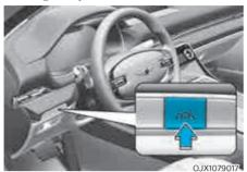
With the Engine Start/Stop button in the ON position, press the Lane Safety button located on the instrument panel to turn on Lane Keeping Assist. The white indicator light will illuminate on the cluster.
