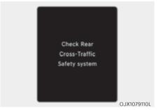
When Rear Cross-Traffic Safety system is not working properly, the 'Check Rear Cross-Traffic Safety system' warning message will appear on the cluster, and the system will turn off automatically or the system will be limited. Have the system inspected by an authorized retailer of Genesis Branded products.
