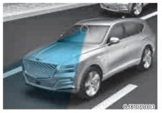
The front view camera is a sensor that detects the front road. If the windshield or the front view camera is covered with snow, rain or foreign matters, the data collected by the camera is limited due to the degradation of the camera's performance. Always keep the front view camera clean.
