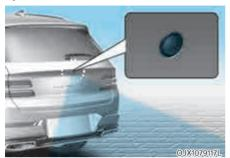
The rear view camera is used as a detecting sensor to detect pedestrians. If the camera lens is covered with foreign material, such as snow or rain, it may adversely affect camera performance and Reverse Parking Collision-Avoidance Assist may not operate normally. Always keep the camera lens clean.
