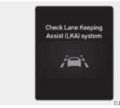
When Lane Keeping Assist is not working properly, the 'Check Lane Keeping Assist (LKA) system' warning message will appear and the yellow indicator light will illuminate on the cluster. If this occurs, have the system inspected by an authorized retailer of Genesis Branded products.
