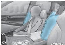
Your vehicle is equipped with a side air bag in each front and outboard second row seat. Additionally, a front center air bag is provided in the inboard side of the driver seatback. The purpose of the air bag is to provide the vehicle's additional protection than that offered by the seat belt alone.
