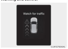
Collision warning when exiting vehicle
