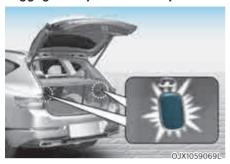
The lamp turns on when the liftgate is opened.
