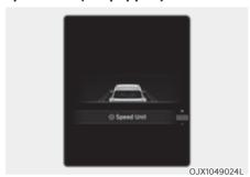
When the Speed Unit menu is selected, press the OK switch on the steering wheel. You can change the speed unit setting between MPH and km/h for the cluster.
