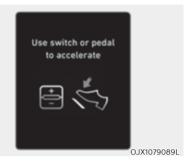
In traffic, your vehicle will stop if the vehicle ahead of you stops. Also, if the vehicle ahead of you starts moving, your vehicle will start as well. In addition, after the vehicle has stopped and a certain time have passed, the 'Use switch or pedal to accelerate' message will appear on the cluster. Depress the accelerator pedal or push the + switch, - switch or III switch to start driving.
