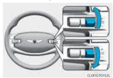
To resume Manual Speed Limit Assist after the system was paused, push the +, -, || 5 switch.
