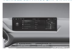
Vehicle Settings in the infotainment system provides user options for a variety of settings including door lock/ unlock features, convenience features, driver assistance settings, etc.
