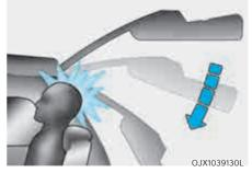
Be careful when closing the tailgate with passenger's seated on the third row seat. If the passenger's head is not properly against an adjusted head restraint or a tall person is seated, the tailgate may hit the passenger's head, which could cause injury.
