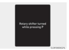
This message is displayed when the shift dial is rotated while pressing the P button.
