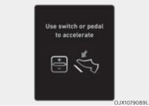
When Highway Driving Assist is operating, your vehicle will stop if the vehicle ahead of you stops. Also, if the vehicle ahead of you starts moving within 30 seconds after the stop, your vehicle will start as well. In addition, after the vehicle has stopped and 30 seconds have passed, the 'Use switch or pedal to accelerate' message will appear on the cluster. Depress the accelerator pedal or push the + switch, - switch or II' witch to start driving.
