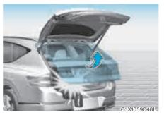
During power opening or closing if the power liftgate senses any obstacle, the power liftgate will stop and move in the opposite direction.
