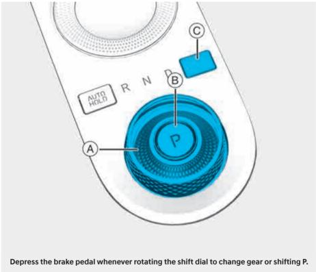
[A]: Rotary shifter (Rotary gear shift dial), [B]: Park button, [C]: Cap-cover
