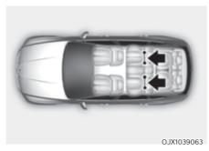
LATCH anchors have been provided in the left and right outboard rear seating positions. Their locations are shown in the illustration.
