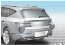
[1]: Front view camera, [2]: Rear corner radar Refer to the picture above for the detailed location of the detecting
