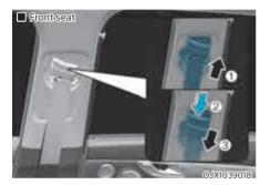
To adjust the height of the seat belt anchor, lower or raise the height adjuster into an appropriate position.
