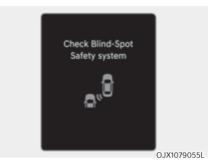
When Blind-Spot Safety system is not working properly, the 'Check Blind-Spot Safety system' warning message will appear on the cluster, and the system will turn off automatically or the system will be limited. Have the system inspected by an authorized retailer of Genesis Branded products.
