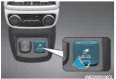
The AC inverter supplies 115 volts (150 watts) electric power to operate electric accessories or equipment.
