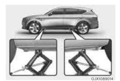
7. Place the jack at the designated jacking position under the frame closest to the tire you are changing. The jacking positions are plates welded to the frame with two notches. Never jack at any other position or part of the vehicle. Doing so may damage the side seal molding or other parts of the vehicle.
