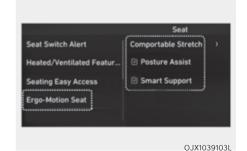
Select 'Ergo-Motion Seat' from the infotainment system's Settings menu to select and set up supplemental functions for the driver.
