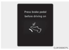
Press brake pedal before driving on When the gear is shifted from N (Neutral) to R (Reverse), D (Drive) or Manual shift mode without the brake pedal depressed, a message will appear on the cluster LCD display. To activate auto start, depress the brake pedal.
