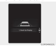
When Head-Up Display menu is selected, press the OK switch on the steering wheel. You can select or deselect head-up display by pressing the OK switch.
