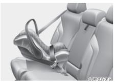
Rearward-facing Child Restraint System A rearward-facing Child Restraint System provides restraint with the seating surface against the back of the child.
