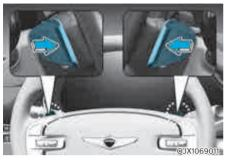
The paddle shifter allows the driver to shift gear without taking one's hands off the steering wheel.
