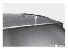
If the LED lamp (1) does not operate, have the system inspected by an authorized retailer of Genesis Branded products.
