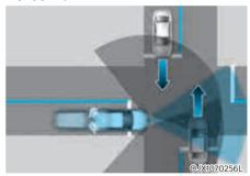
Junction Crossing function will help avoid a collision with oncoming vehicles on the left or right side when crossing an intersection by applying emergency braking.
