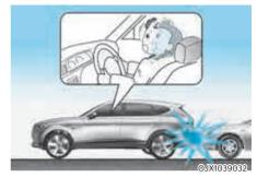
Front air bags are not designed to inflate in rear collisions, because occupants are moved backward by the force of the impact. In this case, inflated air bags would not provide any additional benefit.
