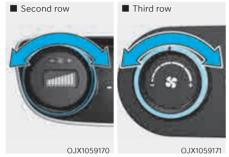
The fan speed can be set to the desired speed touching the x or x icon, or by turning the fan speed control knob.
