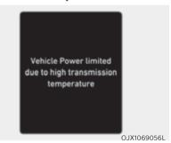
This message is displayed when the transmission oil temperature is high.
