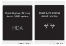
When Highway Driving Assist or Highway Lane Change function is not working properly, the 'Check Highway Driving Assist (HDA) system' or 'Check Lane Change Assist function' warning message will appear, and the Awarning light will illuminate on the cluster. Have the system inspected by an authorized retailer of Genesis Branded products.
