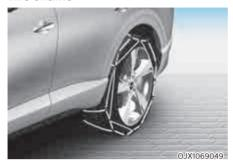
Since the sidewalls of radial tires are thinner than other types of tires, they may be damaged by mounting some types of tire chains on them. Therefore, the use of snow tires is recommended instead of tire chains. If tire chains must be used, use genuine Genesis parts and install the tire chain after reviewing the instructions provided with the tire chains. Damage to your vehicle caused by improper tire chain use is not covered by your vehicle manufacturer's warranty.
