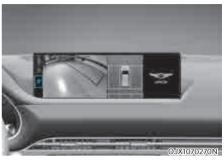
You can change Surround View Monitor settings by pressing the setup icon (a) on the screen while the system is operating, or select 'Driver Assistance → Parking Safety → Camera Settings' from the Settings menu while the Engine Start/Stop button is in the ON position.
