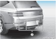
[1]: Rear view camera, [2]: Rear ultrasonic sensors Refer to the picture above for the detailed location of the detecting sensors.
