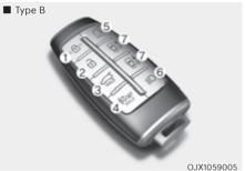
Your Genesis Branded Vehicle uses a Smart Key, which you can use to lock or unlock the driver and passenger doors or the rear liftgate.
