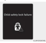
When electronic child safety lock does not work even though the button is pressed, the message will be displayed and an alarm will sound. If this occurs, have the vehicle inspected by an authorized retailer Genesis Branded products.
