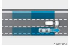
Blind-Spot Collision-Avoidance Assist will help detect and inform the driver that a vehicle is in the blind spot.
