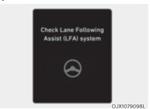
When Lane Following Assist is not working properly, the 'Check Lane Following Assist (LFA) system' warning message will appear on the cluster. If this occurs, have the system inspected by an authorized retailer of Genesis Branded products.
