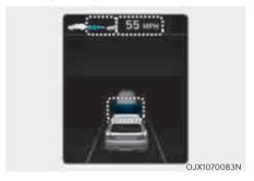
If you want to speed up temporarily when Smart Cruise Control is on, depress the accelerator pedal. While the speed is increasing, the set speed, distance level and target distance will blink on the cluster.
