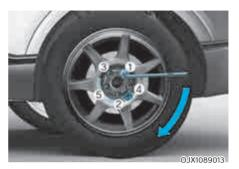
16. Use the wheel lug wrench to tighten the wheel bolts in the order shown. Double-check each wheel bolts until they are tight. After changing tires, have an authorized retailer of Genesis Branded products tighten the wheel bolts to their proper torque as soon as possible. The wheel bolt should be tightened to 101~116 lbf.ft (14~16 kgf.m).
