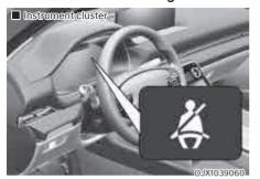
As a reminder to the driver, the seat belt warning light will illuminate for approximately 6 seconds each time the Engine Start/Stop button is in the ON or START position regardless of belt fastening.
