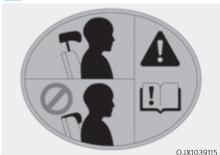
When sitting on the rear seat, do not adjust the height of the head restraint to the lowest position.
