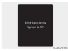
When the engine is restarted with the system off, the 'Blind-Spot Safety System is Off' message will appear on the cluster.
