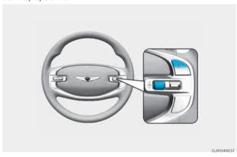
The LCD display modes can be changed by using the control switches.
