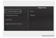
From the infotainment system settings menu, select 'Setup → Vehicle → Digital Key → Enable Digital Key'.
