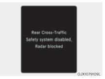
When the rear bumper around the rearside radar or sensor is covered with foreign material, such as snow or rain, or installing a trailer or carrier, it can reduce the detecting performance and temporarily limit or disable Rear Cross-Traffic Safety system.
