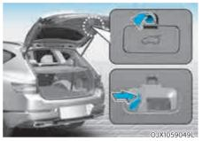
To unlock and open the liftgate manually from inside the luggage compartment, perform the following procedure:
