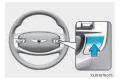
Press and hold Driving Assist MODE button at the desired speed. The Speed Limit (MLIMIT) indicator will illuminate on the cluster.
