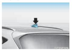
The shark fin antenna will receive AM, FM broadcast and SXM channel signals and transmit data.
